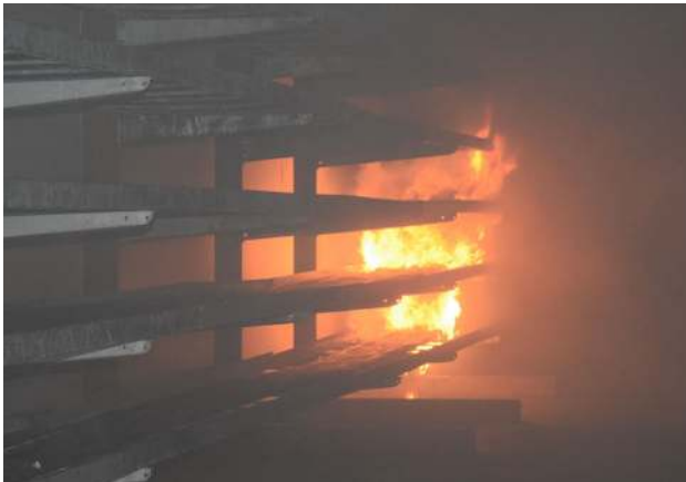
Fig. 2 Cable tunnel fire test
