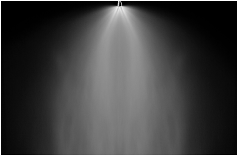
Fig. 1 K6 nozzle water spray
